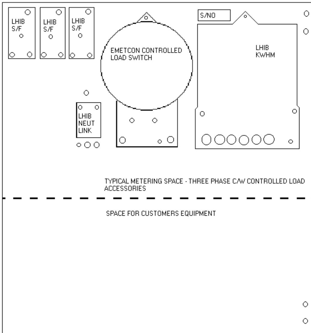
Figure 3 - Typical Three Phase Meter Panel Layout
