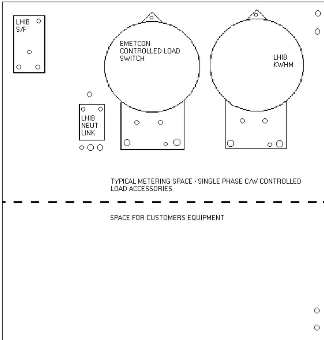
Figure 2 - Typical Single Phase Meter Panel Layout
