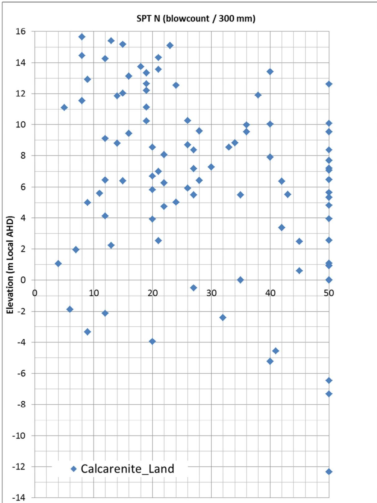
Figure 9-4 SPT N Blow counts in Calcarenite. Values were entered as 1 if less than 1 and 50 if more than 50.
