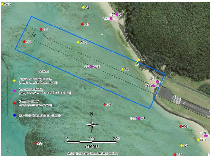
**Figure 7-9 Sediment Samples – extracted from Coastal Study 2014 (sizes in microns) – Georeferenced by AECOM**
