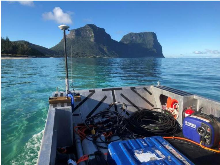
Figure 12-26 Marine Seismic Refraction Set up
