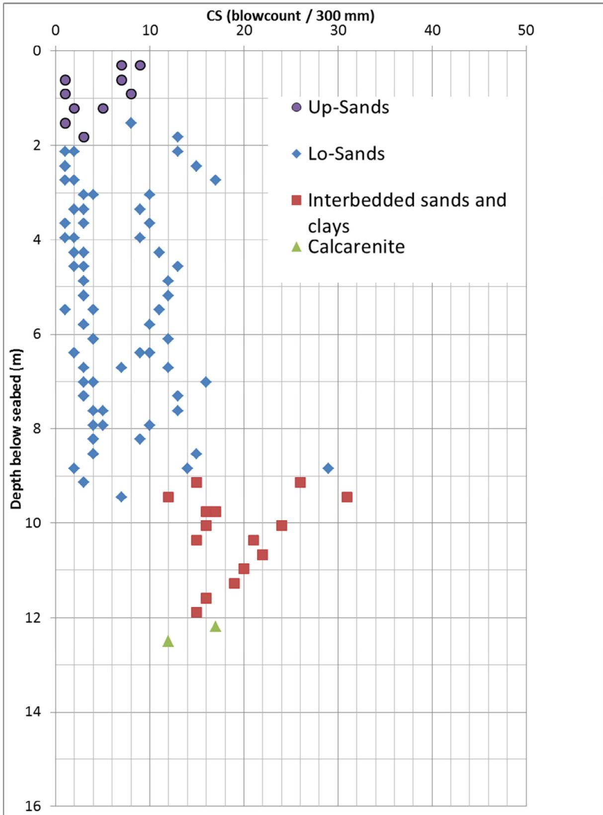
Figure 9-3 CS Blow counts (marine boreholes only) – values were entered as 1 if less than 1 and 50 if more than 50.
