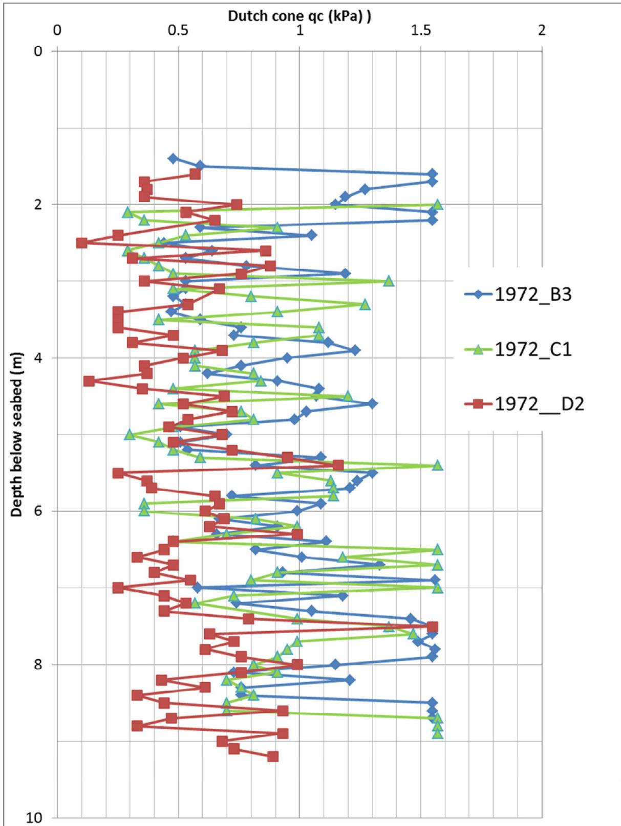
Figure 9-5 Non-normalised cone end resistance
