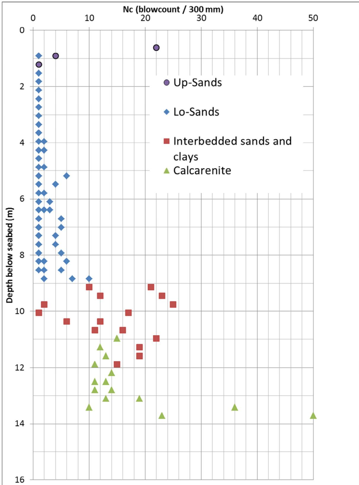
Figure 9-2 Nc Blow counts (marine boreholes only) – values were entered as 1 if less than 1 and 50 if more than 50.
