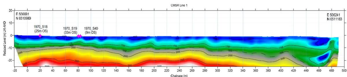
Figure 10 Seismic Refraction Survey - Line 1 (along Runway)
