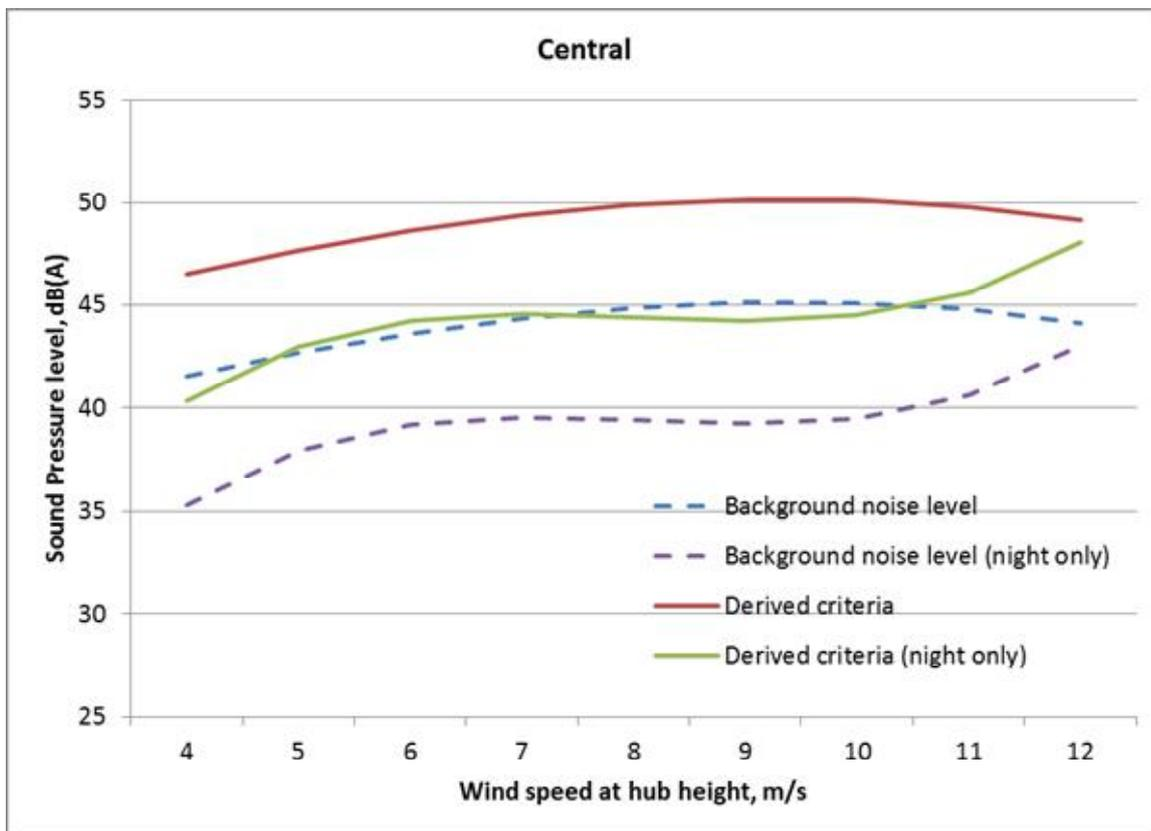
Figure 4-3 Derived noise criteria for western coastal receivers
