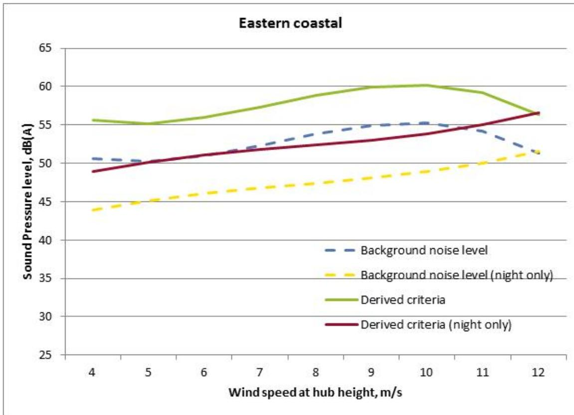
Figure 4-2 Derived noise criteria for central / Joy's Shop area-centre receivers
