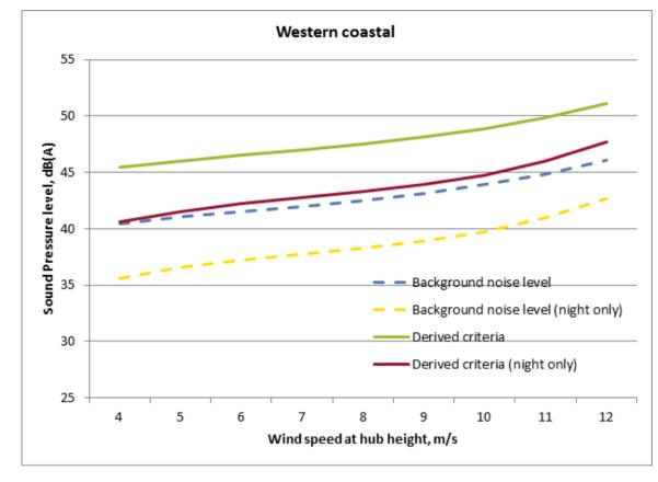
Figure 4-3 Derived noise criteria for western coastal receivers
