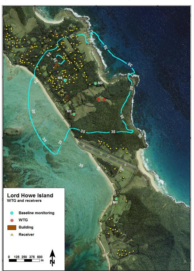
Figure 3-1 Lord Howe Island WTG locations and sensitive receivers for hub height wind speed12 m/s
