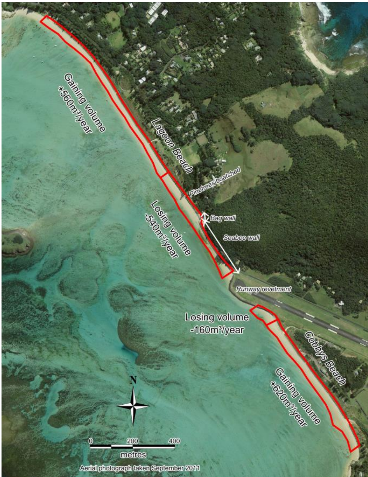
Figure ES1: Summary of long term (1965 to 2011) sand volume changes at Lagoon Beach and Cobbys Beach
