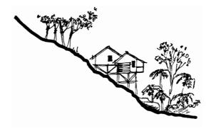
Excessive depths of cut and fill will not be acceptable for site levelling. Appropriate solutions can include split level housing stepping down the site.
