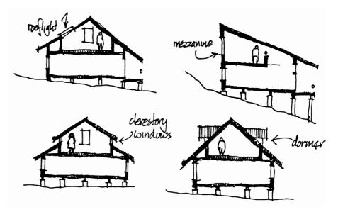
Avoid excessive elevation of floor levels on visually prominent, steeper slopes – buildings are better planned to step down slopes wherever possible.
