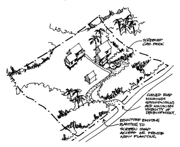
Try to avoid a long access road, or one which requires significant cut or fill, or which crosses a watershed or creek line. If possible, relocate the building to another part of the site to reduce access impacts.
