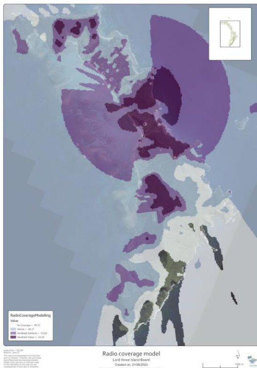
Figure 7 – Current VHF radio coverage (estimated)
