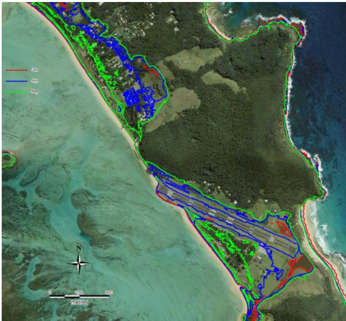
Figure 7-3 3m, 4m and 5m AHD contours along the Lagoon shoreline (Haskoning Australia, 2014)
