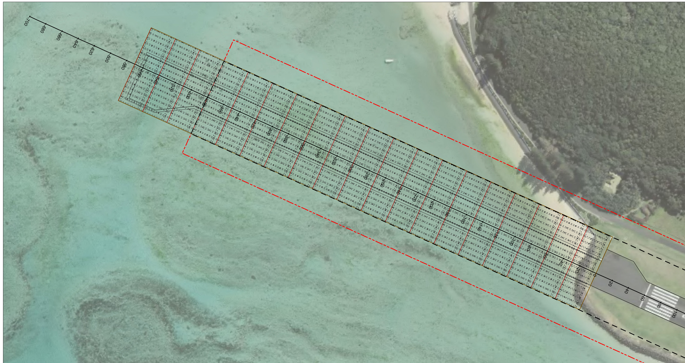
FIGURE 3-3 RUNWAY EXTENSION OPTION – DECK ON PILES
