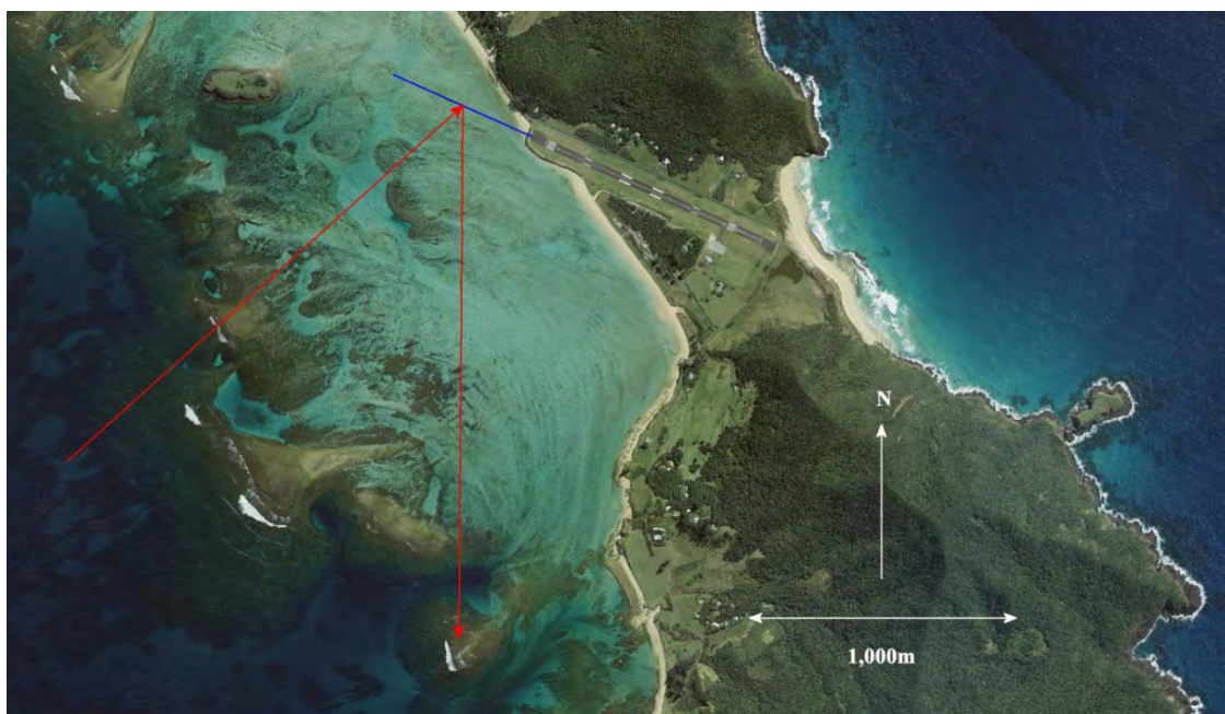
Figure 20: Reflected angle of vector-average offshore wave direction off extended runway (ignoring wave refraction over Lagoon bed)
