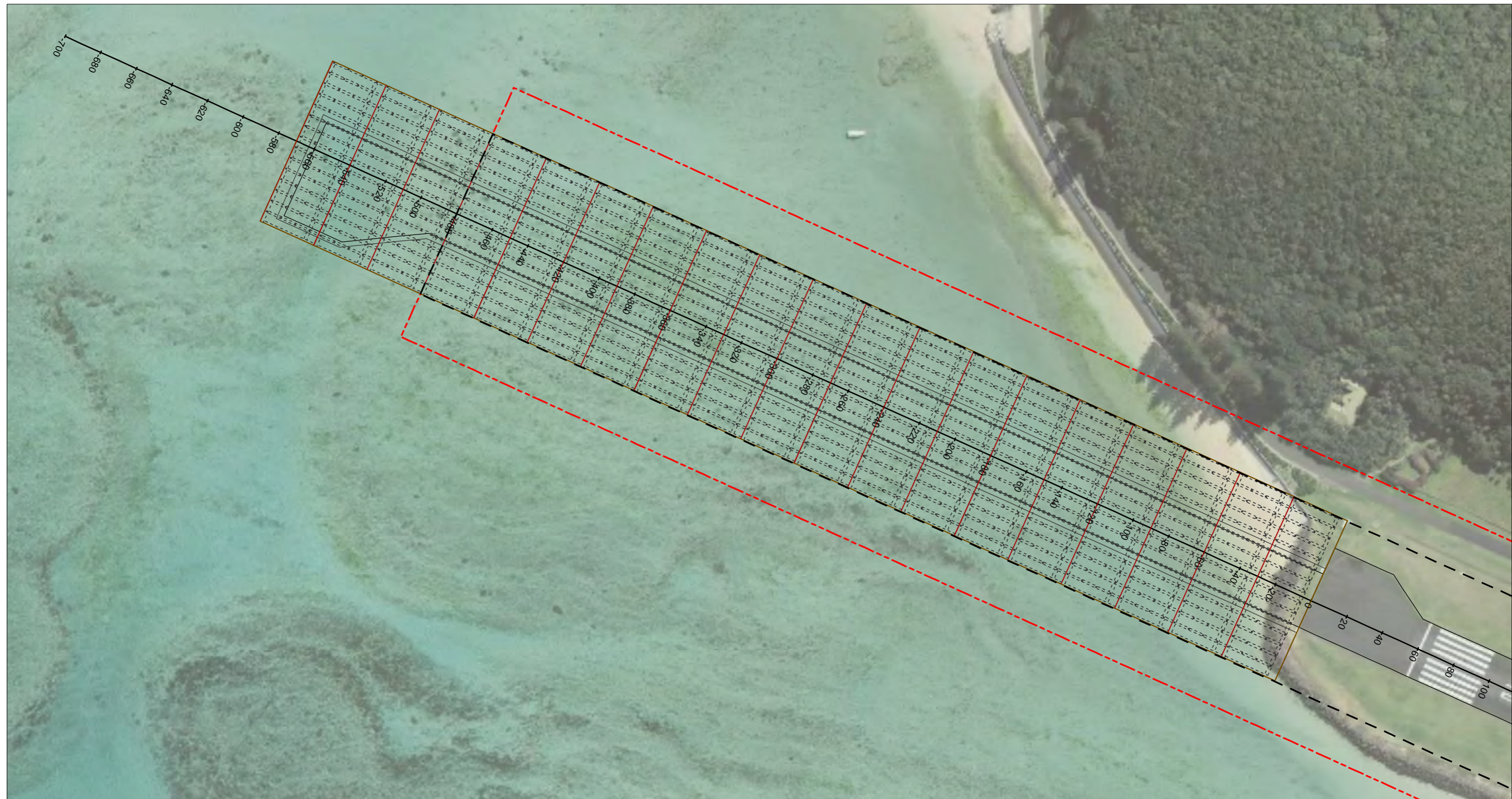
FIGURE 3-3 RUNWAY EXTENSION OPTION – DECK ON PILES
