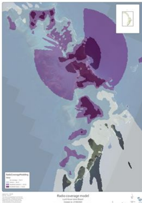
Figure 7 – Current VHF radio coverage (estimated)
