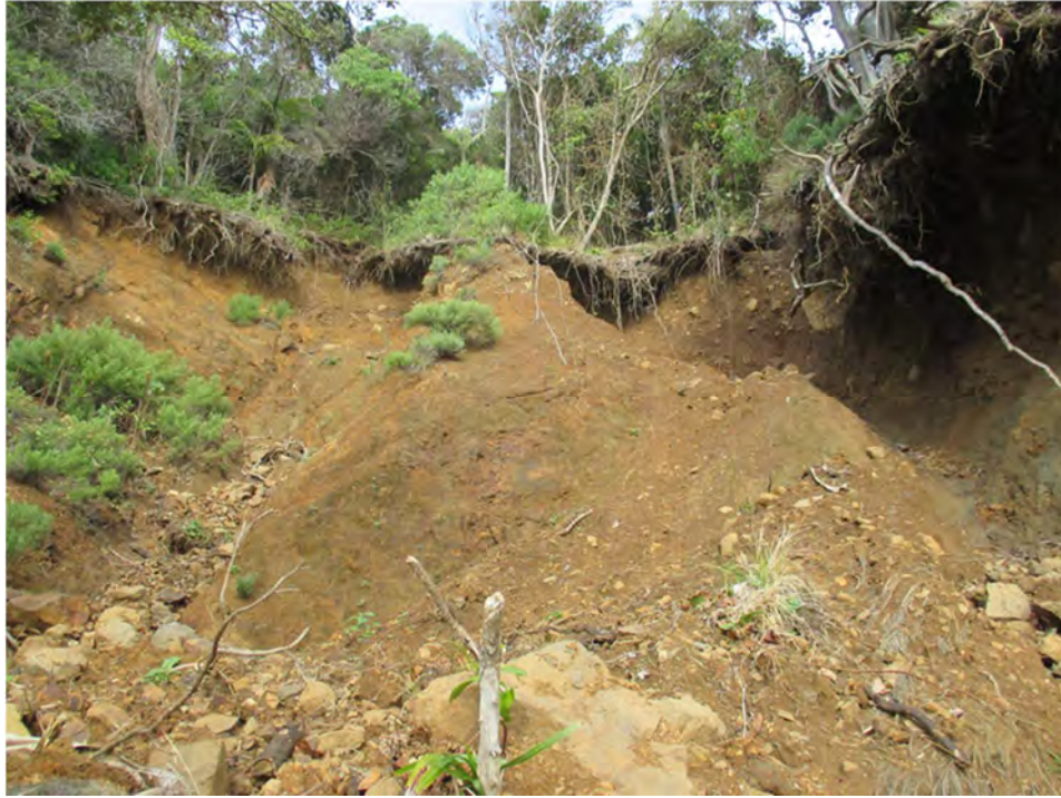
Photo 3- Main backscarp area showing two scour channels incised into weathered bedrock (weathered soft dyke materials?) with overlying mantle of colluvium exposed within the back face of the scarp and transported boulder debris in the foreground.
