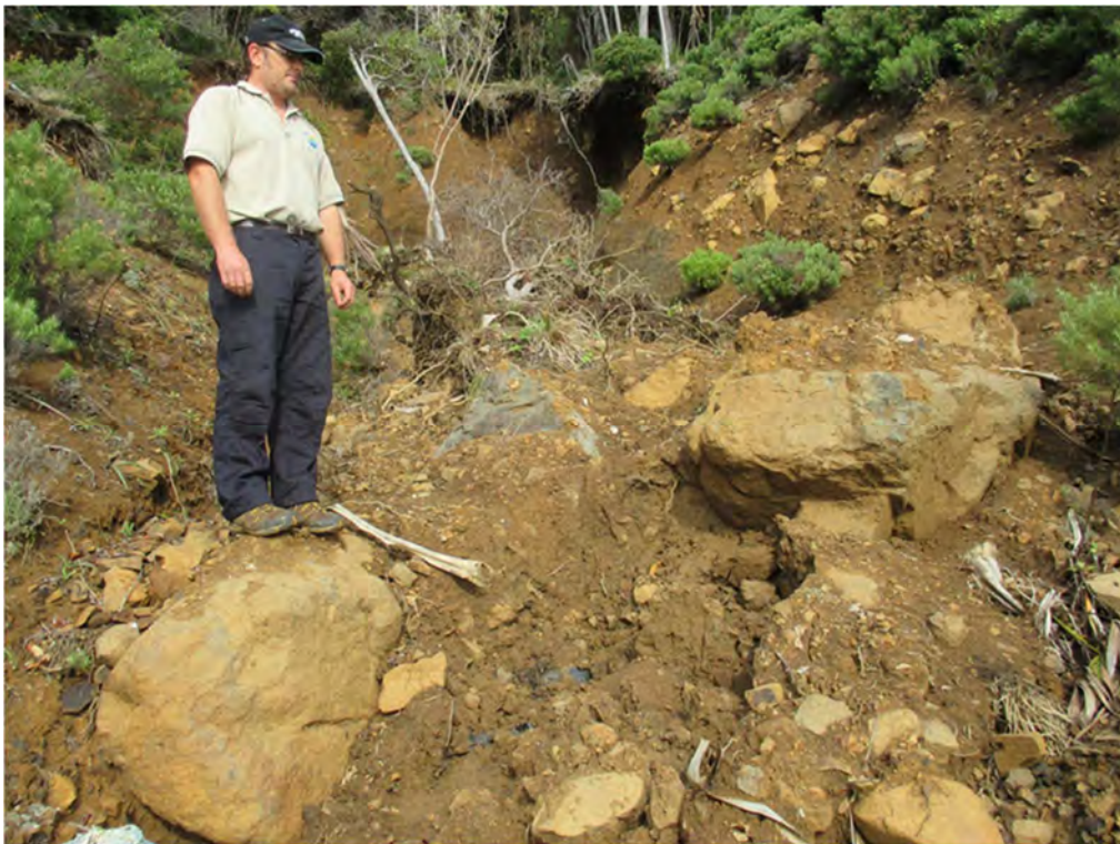
Photo 5; Exposure of north west face of main channel of slide showing upper colluvial mantle containing large boulders and underlying weathered bedrock in left bottom corner of photo.
