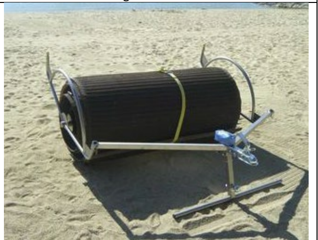
Matting storage and deployment roller
