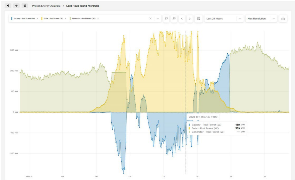
Figure 1 – Electricity generation for Lord Howe Island on 11 November 2020 (a typical day)
