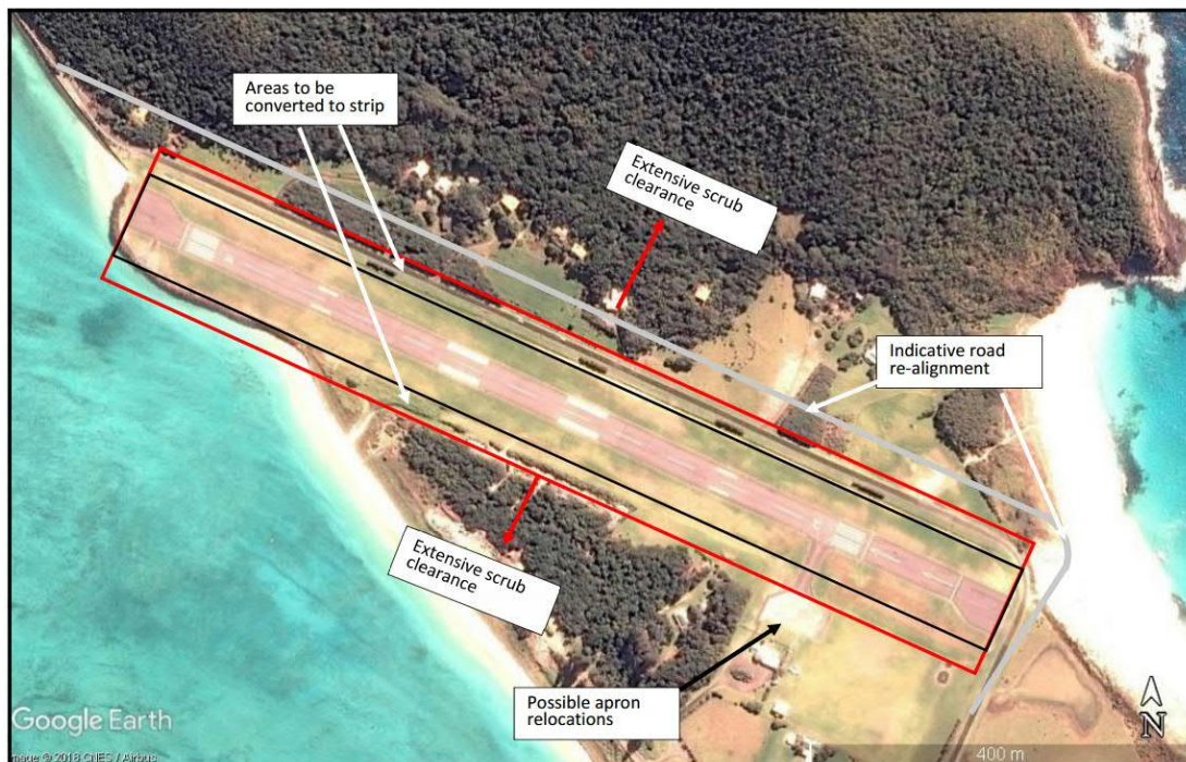
Figure 12 Potential effects of a 140m runway strip at LDH
