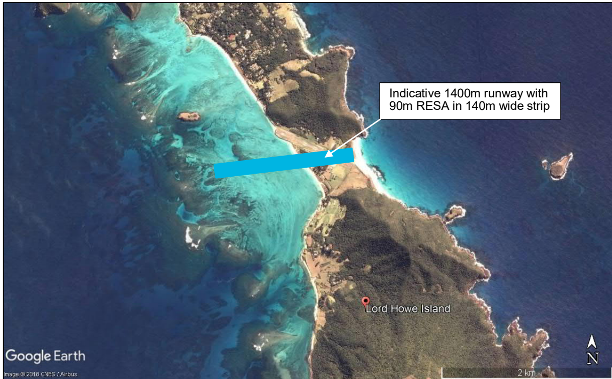
Figure 43 Optimal operational runway realignment
