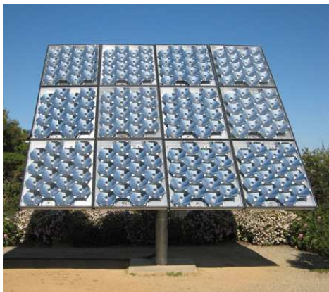
Figure 4: Concentrating PV Array – SolFocus
