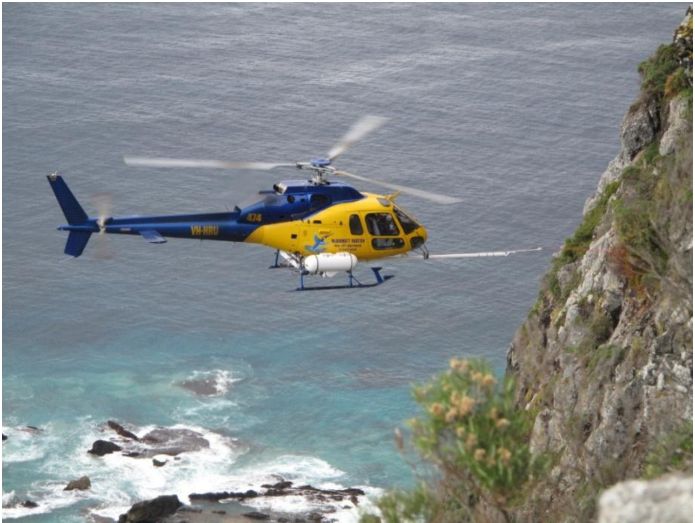
Figure 5 The helicopter-mounted lance-spray unit from McDermott Aviation in action.
