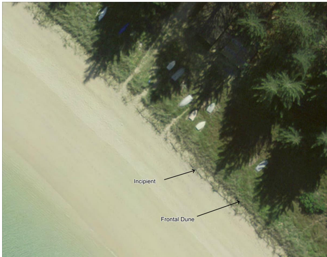
Figure B12: Example definition of incipient and frontal dune sand/vegetation interfaces
