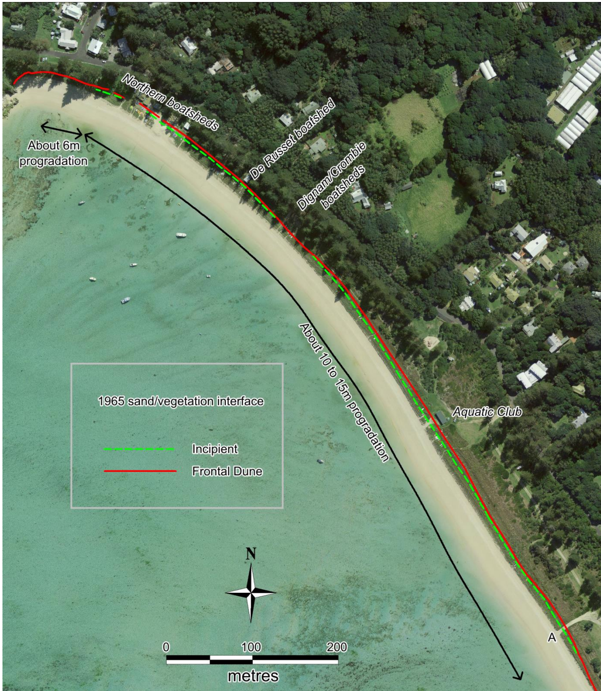
Figure B13: Position of 1965 sand/vegetation interfaces at northern end of Lagoon Beach overlaid on 2011 aerial photograph
