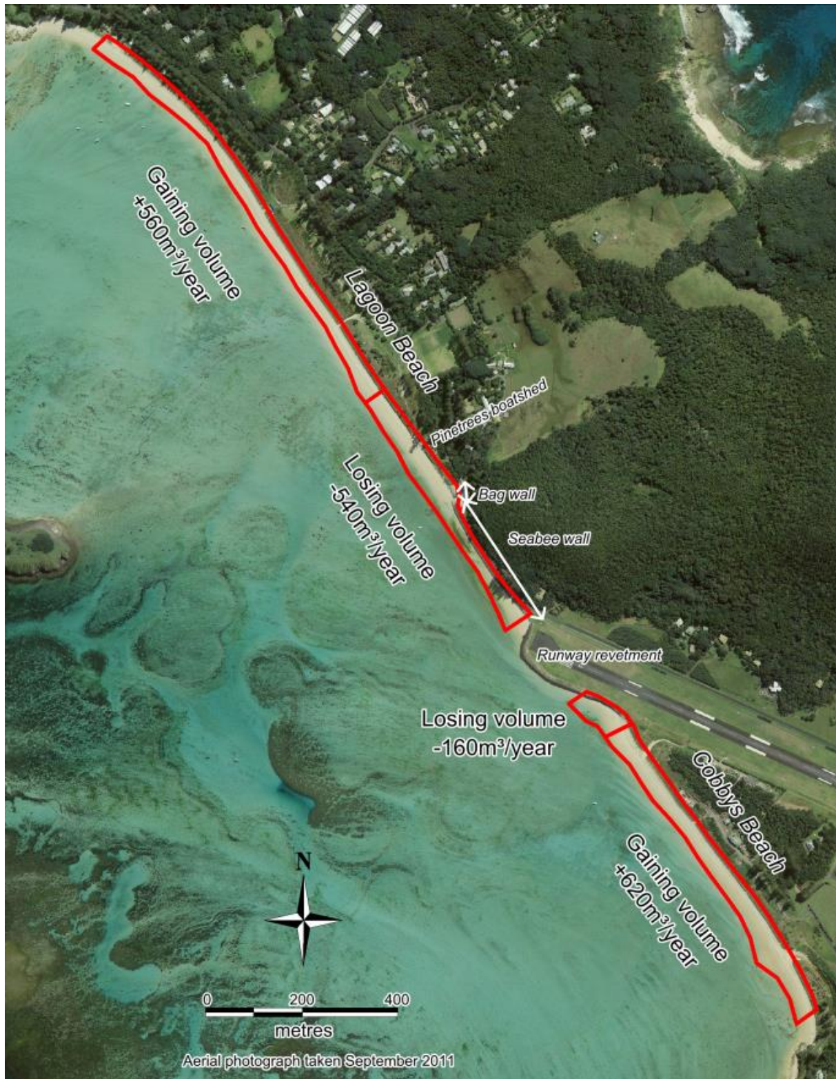
Figure 12: Summary of long term (1965 to 2011) sand volume changes at Lagoon Beach and Cobbys Beach
