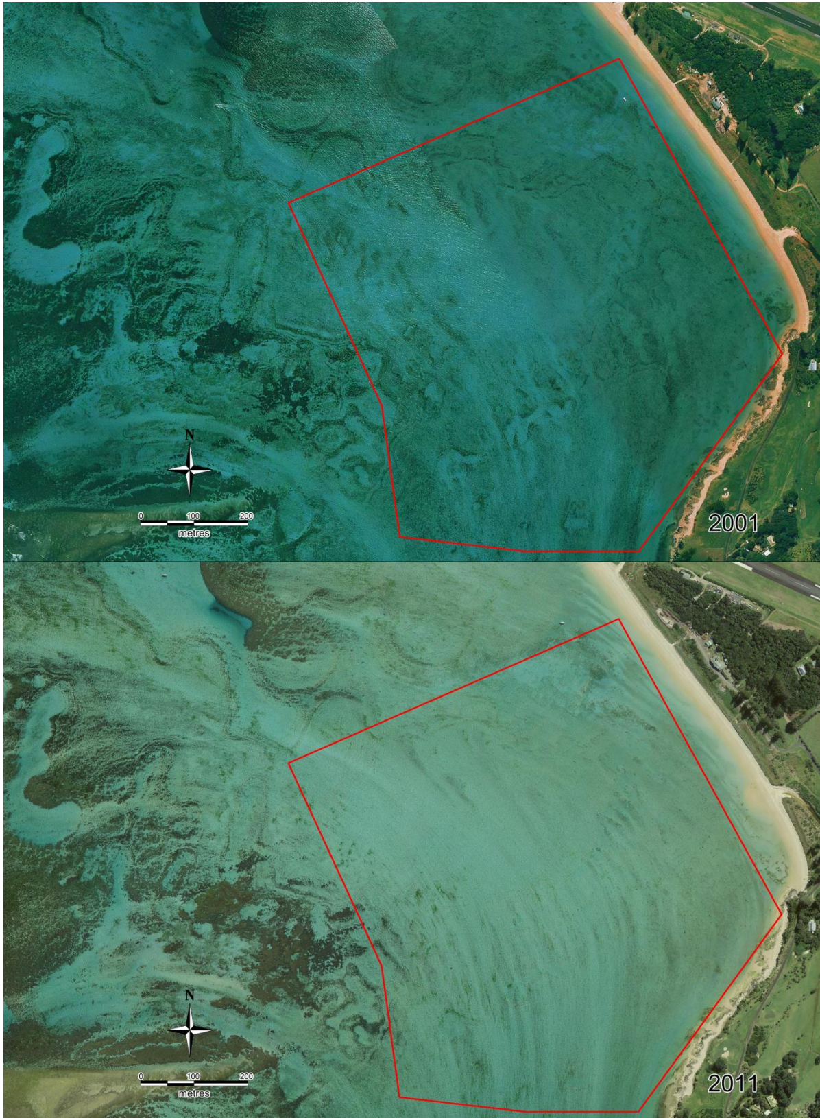
Figure 14: Evidence of sediment smothering reef areas at Cobby's Beach (2001 top, and 2011 bottom), with main area of potential smothering within red box
