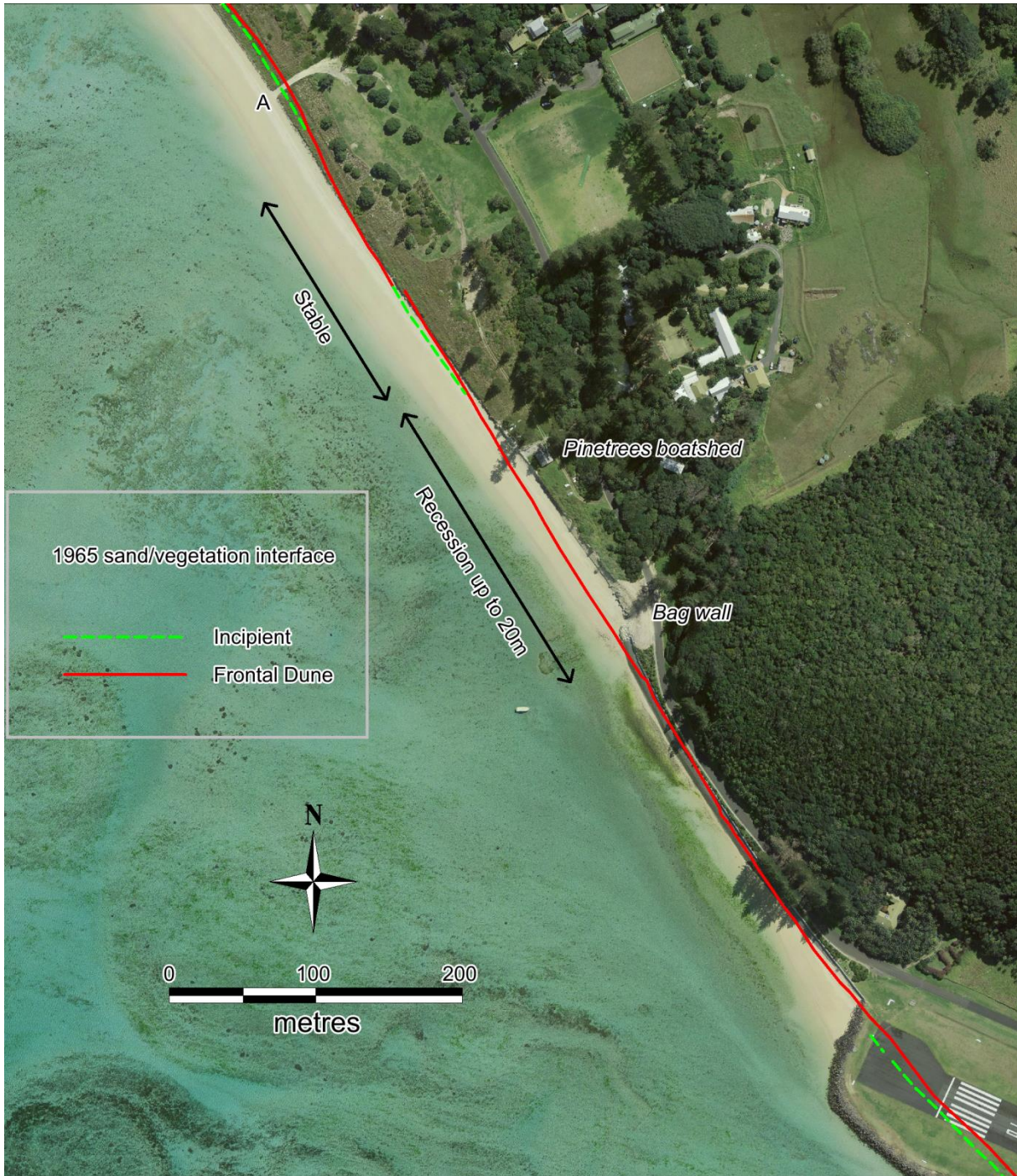
Figure B14: Position of 1965 sand/vegetation interfaces at southern end of Lagoon Beach overlaid on 2011 aerial photograph
